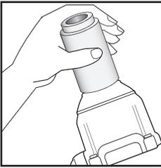
Slide the Fab-Lok setting tool over the nose of a DEWALT versa-clutch screw gun and tighten the set screw with the included hex key. The torque setting of the tool should be adjusted to ensure a proper installation without overdriving.
